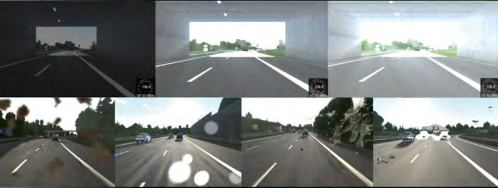
Camera Sensor Exposure & contamination Simulation
